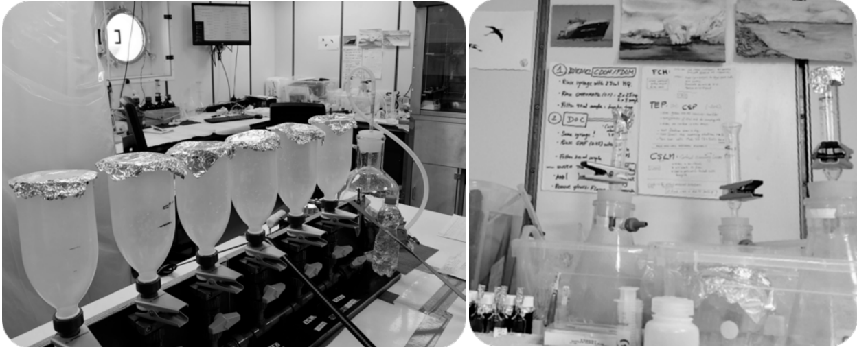
Fig. 5.11 General overview of the wet lab during MSM85, showing on the first plain the filtration track used for collecting POC/PN and chlorophyll a samples. The right panel is a close up of the area where TEP, CSP and CLSM were filtered and stained. Measurements for CDOM, FDOM, DOC and Flow Cytometry were also performed between the area on the right panel and under the fume hood.
